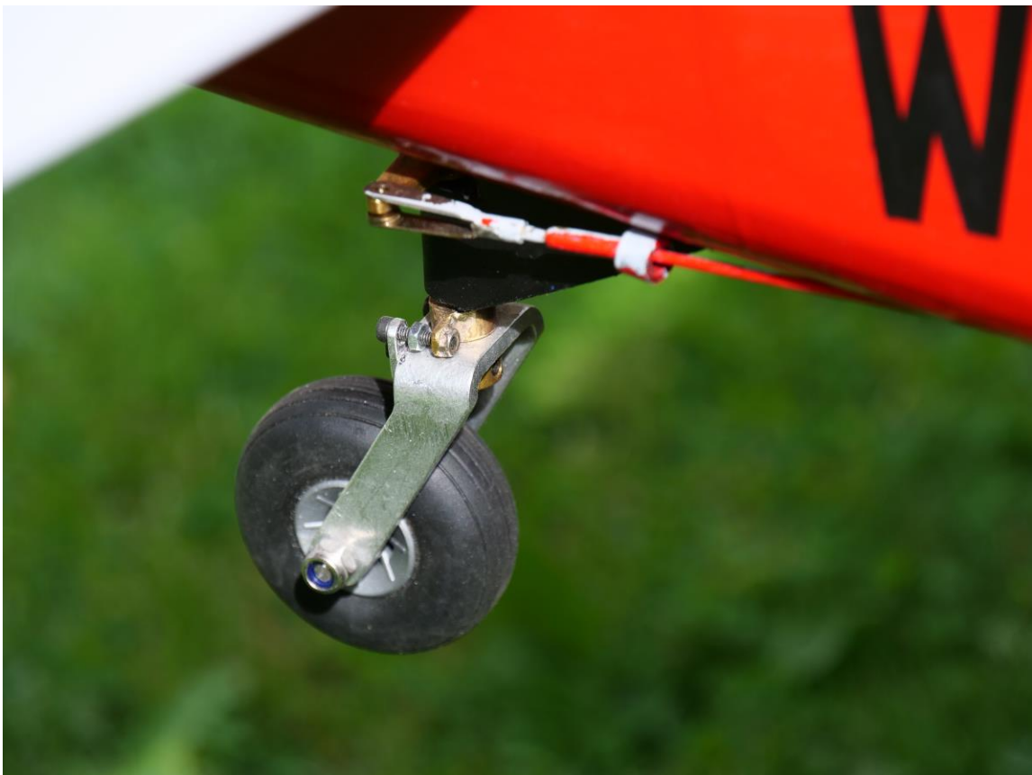
Adjustable tail wheel mechanism
