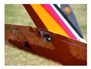
mechanism. Both the Acrowot and release mechanism receivers were simultaneously "bound" to the transmitter but making sure that the channel used for the tow release was not being used by the tug. The tow release was attached under the Acrowot fuselage as shown.
